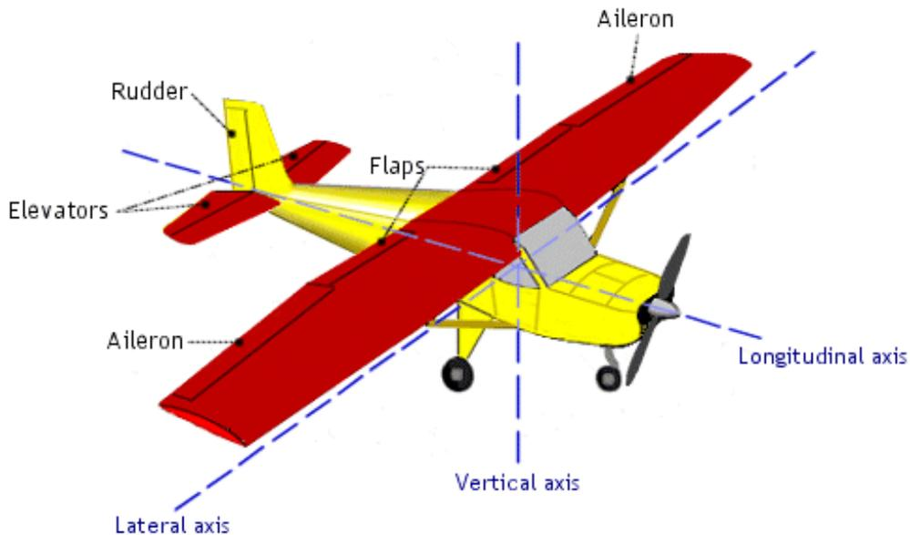
Imagine three lines running through an aeroplane and intersecting at right angles at the aeroplanes centre of gravity.
